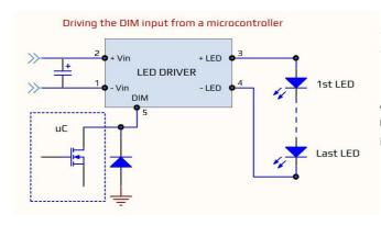
Driving the DIM input from a microcontroller
