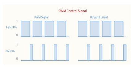
A preferred method is using pulse width modulation (PWM). As shown at next, the output current is adjusted by applying a PWM signal to the DIM input. By varying the signal duty cycle the average output current is adjusted up or down. To avoid visible flicker, the PWM signal should be greater than 200 Hz.
