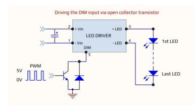
Driving the DIM input via open collector transistor
